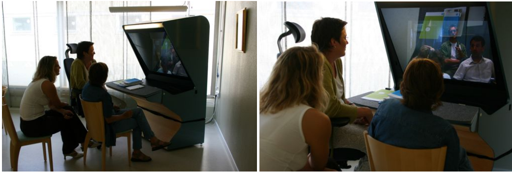
124. As opposed to the previous example, the camera used in the 'Mediated Unemployment Services' was hidden beneath the desktop of this piece of furniture. Two reflective devices were used in this case. A small conventional mirror near the camera reflected what the camera captures in a larger semi-transparent mirror. A plasma display was placed vertically behind the mirror. The furniture was height adjustable, allowing also disabled persons to use the remote meeting-place. (Furniture designed for the 'Mediated Unemployment Services')
