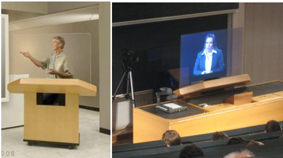
130. Digital Video Enterprise holds several patents for teleprompter applications that enable mutual gaze. Here, a telepresence podium serves a remote lecturer who is displayed onto a coated sheet of glass, located in a lecture hall. The side view shows how back projection is used. A mirror is used to reflect the captured image onto the glass. Left: from the website of Digital Video Enterprise (DVE 2009). Right: as displayed at KTH in December 2009.
