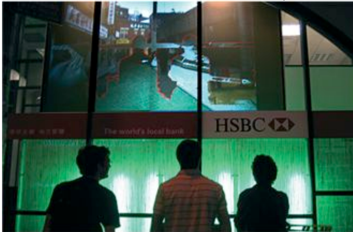
69. A mediated facade for the HSBC bank on Canal Street, NY (2006), by Architects Marisa Yiu and Eric Schuldenfrei. Real-time video and software allows a computer to generate and control masked images, enabling a camera (in a window across the street) to identify the movements of passers-by, by creating an outline of their bodies and then replacing these with time-lapse footage, from, for example, a fish market. The resulting composite images are projected onto the screen, changing its texture and image in real time as people walk by. (Yiu & Schuldenfrei 2006)
