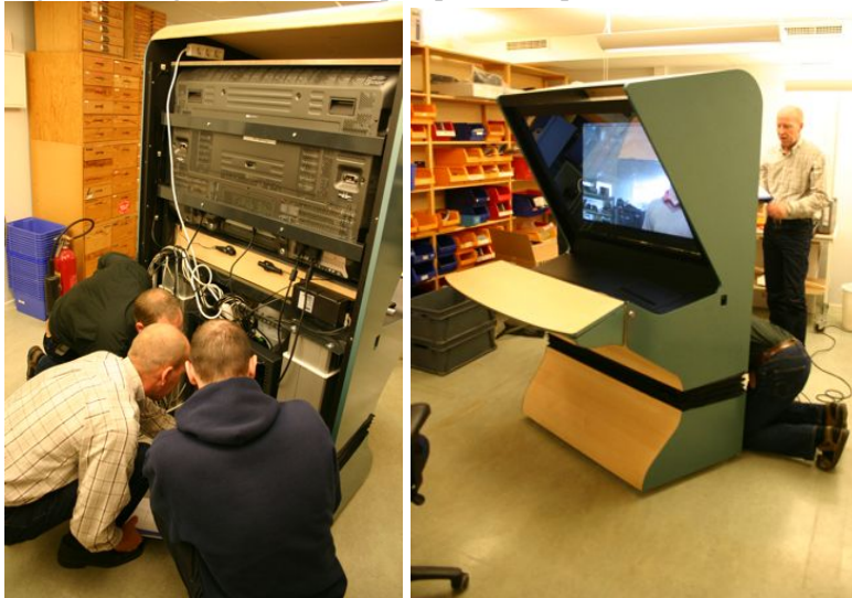
78. On the back of the furniture piece a panel can be removed to allow monitoring of the various equipment that captures, transmits, and represents a remote location.
