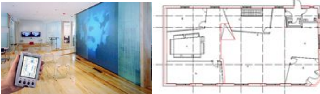
70. Back-projection is used to create ‘interactive wall-paper’ at the Swiss consulate in Massachusetts, US Cameras are placed in several locations, e.g. to the left of the large wall, and between the two displays at the far end, facilitating worldwide, remote interaction. Designs by Convergeo. (Waldvogel & Huang 2000)
