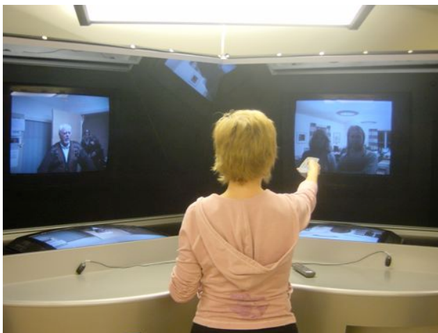
123. Here a slightly different design concept is used. Conventional TV-monitors were placed horizontally (seen resting as an extension of the desktop) and reflected upward onto a semi-transparent beamsplitter placed at 45^\circ . The camera was placed behind the beamsplitter, which had a special coating that allowed the camera to capture the person through its glass, at an approximated eye-height of an adult person. ('Remote Affinity in the Archipelago' design example)
